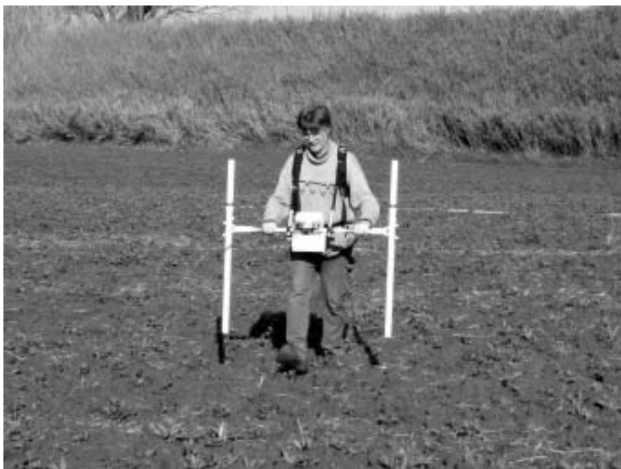
FIG. 12.3. Geophysical survey in progress in 2008 using a Bartington gradiometer. (Portus Project.)
