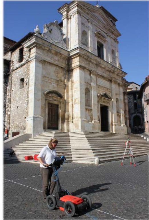
Figure 1: GPR survey data collection in Piazza Santa Maria.
